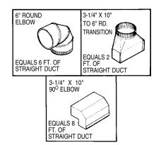
3. The system will operate most efficiently when the ductwork does not exceed 40 feet of equivalent duct. The chart, above, shows equivalent feet of elbows and transitions. The number of feet of straight duct plus the equivalent feet of transitions and/or elbows to be used should equal 40 feet or less.
